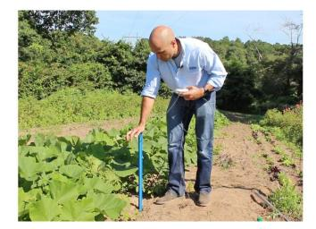
The HOBOnet Multi-Depth Soil Moisture Sensor is a wireless sensor that works with the HOBOnet system to measure soil moisture and soil temperature at multiple depths with a single probe, for fast and easy installation. This durable sensor is available in three probe lengths for measurements from 45 cm (18 in) to 90 cm (35 in) deep.
