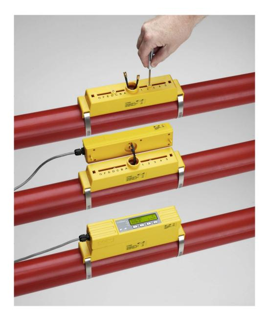
The Micronics U1000MKII-FM is a Fixed, clamp-on, pipe mounted, ultrasonic flow meter, which delivers significant installation savings and non-invasive, dry servicing benefits for pipe sizes ranging from 22mm – 180mm (6") OD.
