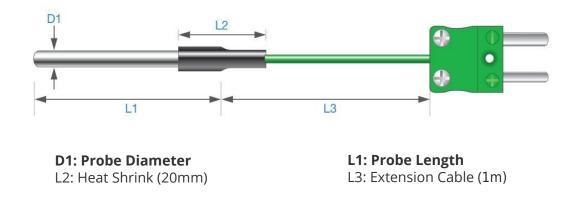
Material sheath 316 stainless steel probe with crimp end seal and fitted with PVC heat shrink for sealing and strain relief. The sensor is supplied with **1 metre of PFA Insulated lead** and Mini Plug. A range of accessories including extension cables, connectors, pockets, thermowells and adjustable compression fittings are available for this product.
