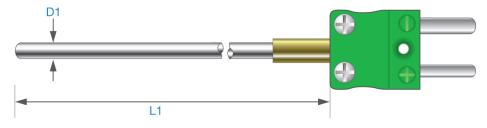
D1: Probe Diameter L1: Probe Length
