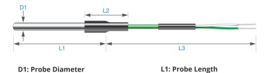
Material sheath 316 stainless steel probe with crimp end seal and fitted with PVC heat shrink for sealing and strain relief. The sensor is supplied with **1 metre of PFA Insulated lead**.
