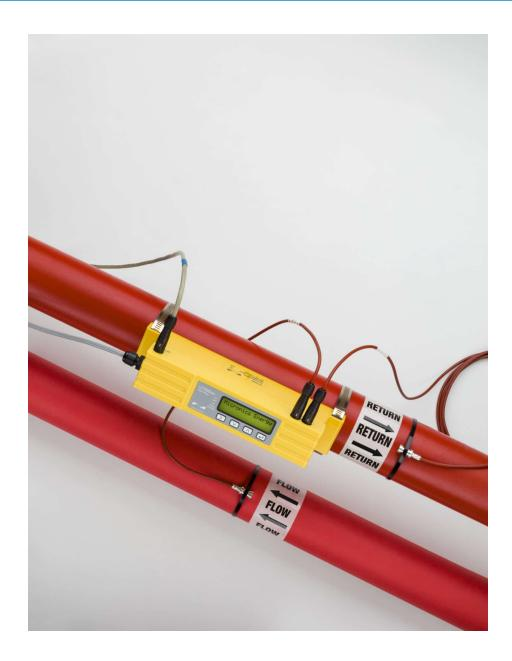
The U1000MKII-HM is an ultrasonic clamp-on thermal, heat/ energy meter that uses ultrasound to measure flow rate and PT100 temperature sensors to measure flow and return temperatures. The U1000MKII-HM displays energy rate and totalised energy with pulse output and communication options, so it can be used as a standalone meter or as an integral part of an aM&T or BEM's system.
