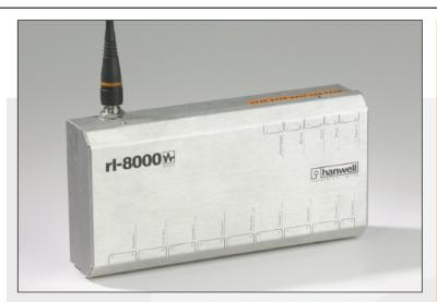
The 8-Zone Flood Alarm is a radio transmitter connected to up to eight highly responsive flood detection cables. These cables can be run along key areas enabling rapid notification of water leakage before serious damage can be done.
