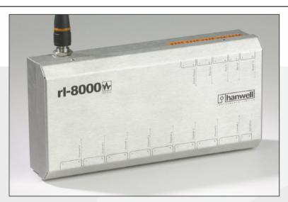
rl8000 radiologgers are a highly flexible solution to a wide variety of low-speed instrumentation problems. The unit offers 8 configurable input channels and a variety of communication options including radio telemetry, TCP/IP and direct wired.
