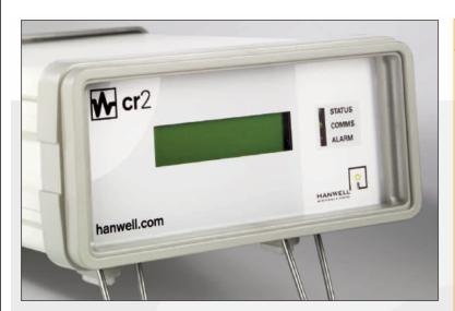
The base station receives and processes signals from Hanwell radio and wired sensors. These sensors communicate at regular short intervals with the cr2, which logs and stores the data pending transfer to a PC for analysis and archival storage. The cr2 also provides an interface for the ms1000 control system.
