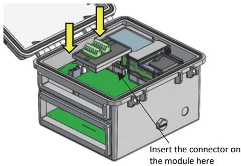
If you are installing an RXW Manager module, plug the cable from the RXW Manager mote into the jack on the module, making sure the cable is inserted through the bottom of the station case. Do not reconnect the power on the station until the mote is plugged in as shown.
