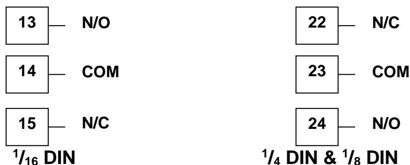
Figure 22. Option Slot 2 - Relay Module
