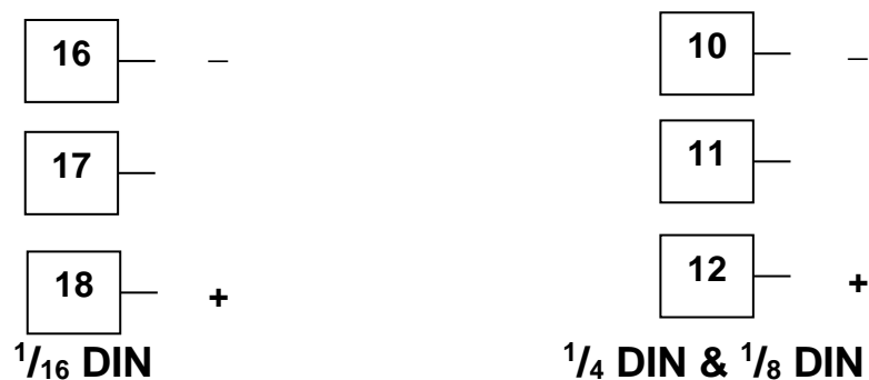
Figure 28. Option Slot 3 - SSR Driver Module
