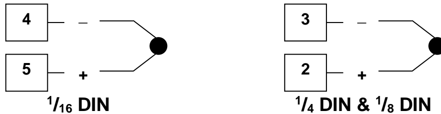
Figure 15. Thermocouple Input Connections
