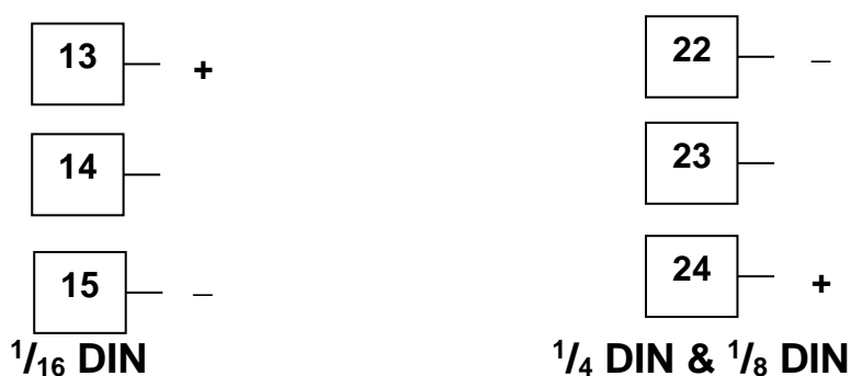
Figure 23. Option Slot 2 - SSR Driver Module
