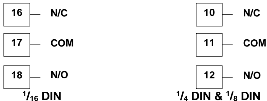
Figure 27. Option Slot 3 - Relay Module
