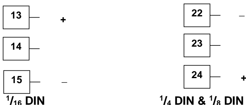
Figure 26. Option Slot 2 - Linear Voltage & mADC module
