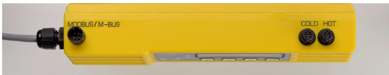
Figure 22 Temperature Sensor connectors on the Electronics Module
