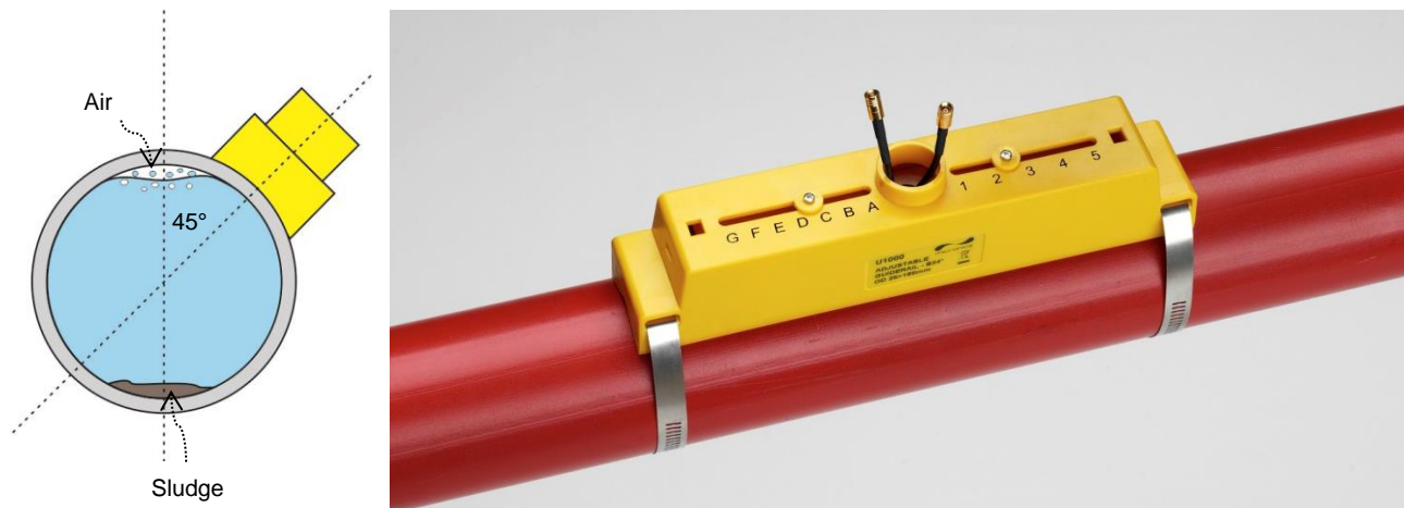
Figure 19 Sensor Assembly clamped at 45^\circ
