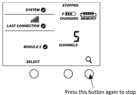
When you are finished adding repeaters and wireless sensors to the network, the total channel count for the module on the station will represent the measurement channels from all motes plus a battery channel for each mote (including repeaters) in the network.
