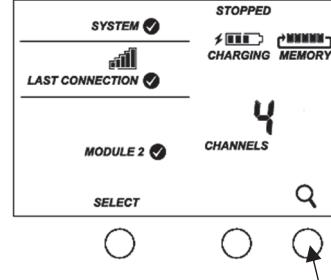
Press this button so the station is ready to have the repeater join the network
