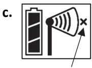
This network connection "x" icon blinks while the repeater completes the registration process, which may take up to five minutes.
