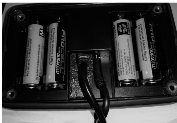
Fig. 1: Cable attached. Foam retainer installed
