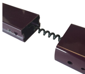
Figure 2. Sensor block/shaft interface
